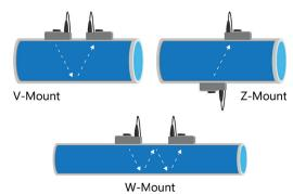
TTFM 6.1 transducers can be mounted on vertical or horizontal pipes, and the pipe must be full. The choice of V, Z, or W mounting method depends on the application and pipe diameter.
