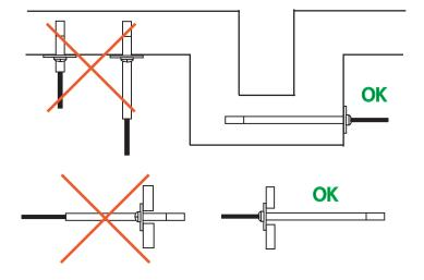
Position the probe so as to prevent the accumulation of condensation water at the level of the sensor leads. Install the probe so that the probe tip is looking downward. If this is not possible, install the probe horizontally.
