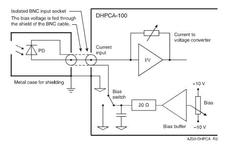
Photo detector biasing through external voltage source
