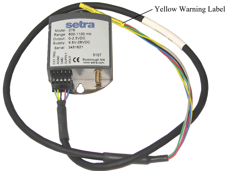
FIGURE 7-3. CS100 and cable with warning label
