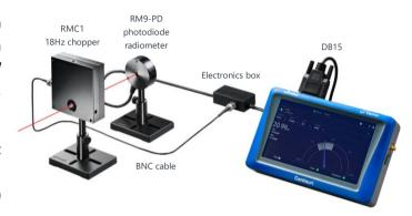
The RMC1 chopper should be mounted with the side marked "THIS SIDE TOWARD SENSOR" facing the RM9-PD. The side of the chopper blade facing this direction has a low emissivity surface. The other side of the blade faces the light source and has an absorptive black coating to minimize stray reflections.
