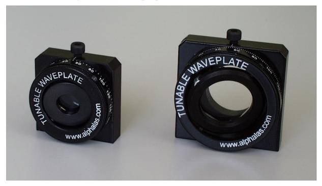
The required phase retardation is achieved by tilting the plates  $0^{\circ}$  -  $45^{\circ}$  using a special tilt holder. Each plate is provided with tuning curves that allow easy adjustment of the desired phase retardation.
