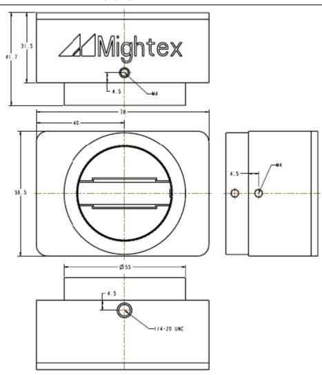
Length x Width x Height: 78(mm) x 42(mm) x 57(mm)
