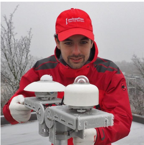
Figure 2 frost and dew deposition: clear difference between a non-heated pyranometer (back) and SR30 with RVH™ technology (front)
