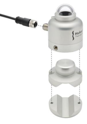
**Figure 3** 'Exploded view' of SR05. The optional ball levelling and tube mount allow for easy installation. The cable (standard 3 m) has an M12-A connector.
