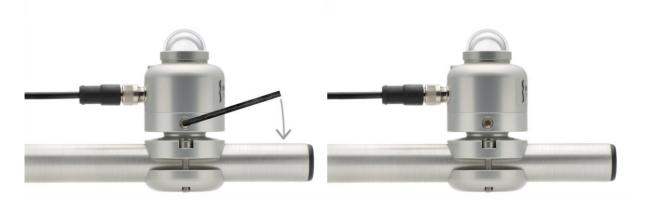
3) tighten set screw to lock ball levelling 4) SR05 is mounted and levelled **Figure 5.4.2.1** Levelling steps for SR05 when mounted on tube mount with ball levelling
