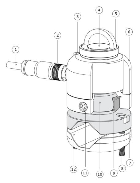
**Figure 2.1** Overview of SR05-A1 (shaded areas in exploded view show ball levelling mount and shim). Numbers 7 to 12 are included when ordering option BL01 or TMBL01:
