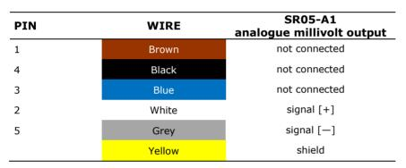
Table 5.5.1 Wiring diagram of SR05-A1
