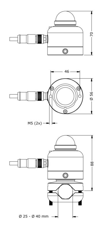
**Figure 3.2.1** Dimensions of SR05 in  $x \ 10^{-3}$  m. The bottom drawing shows the height of SR05 combined with its optional ball levelling mount and the tube diameter required for use with SR05's optional tube mount. M5 mounting bolts and the countersunk set screw require a 4 mm hex key for mounting and levelling.
