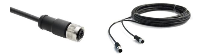
**Figure 8.1.1** On the left the SR05-A1 cable with M12-A female connector on sensor end. The cable is non-stripped on the other end. Its length is 3 metres standard and available in 10 and 20 metres too. On the right Hukseflux extension cable with connector pairs, with male and female M12-A connectors, available in 10 and 20 metres.
