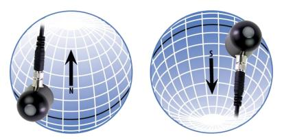
In addition to orienting the cable to point toward the nearest pole, the sensor should also be mounted such that obstructions (e.g., weather station tripod/tower or other instrumentation) do not shade the sensor. **Once mounted, the blue cap should be removed from the sensor.** The green cap can be used as a protective covering for the sensor when it is not in use.
