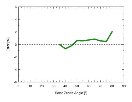
Mean cosine response of five SQ-100X series quantum sensors. Cosine response measurements were made by direct side-by-side comparison to the mean of seven reference SQ-500 quantum sensors.
