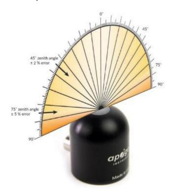
Directional (cosine) response is defined as the measurement error at a specific angle of radiation incidence. Error for Apogee SQ-100x series quantum sensors is approximately  $\pm$  2 % and  $\pm$  5 % at solar zenith angles of 45° and 75°, respectively.
