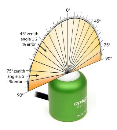
Directional, or cosine, response is defined as the measurement error at a specific angle of radiation incidence. Error for Apogee SE series photometric sensors is approximately  $\pm$  2 % and  $\pm$  5 % at solar zenith angles of 45° and 75°, respectively.
