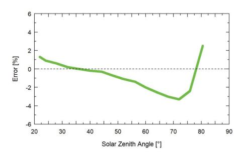
Cosine response measurements were made by direct side-by-side comparison to the mean of four reference SE-100 photometric sensors.
