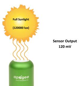
Example of illuminance measurement with an Apogee photometric sensor. Full sunlight yields an illuminance on a horizontal plane at the Earth's surface of approximately 120000 lux. This yields an output signal of 120 mV. The signal is converted to illuminance by multiplying by the calibration factor of 1000 lux per mV.
