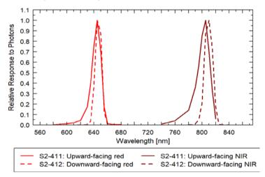
Above: The NDVI sensors have the spectral ranges of 650 nm with 10 nm full-width half-maximum (Red) and 810 nm with 10 nm full-width half-maximum (NIR). The spectral responses can be seen in the graph to the left.
