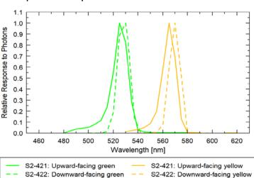
Above: The PRI sensors have the spectral ranges of 532 nm with 10 nm full-width half-maximum (Green) and 570 nm with 10 nm full-width half-maximum (Yellow). The spectral responses can be seen in the graph to the left.
