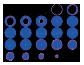
This result shows a LPG-405 laser pulse being stepped through a 4 ns gate window generated by a Photek GM200-3N gate unit on a Photek MCP118 image intensifier. Each step represents an extra 200 ps delay on the laser pulse.
