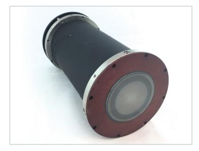
The electron optical design of this tube was adapted from the RCA C 7435 by Ching Lai of Lawrence Livermore National Laboratories in 1986, and was known as the ITT F 4157 tube.
