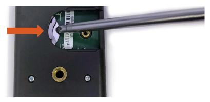
If the battery is difficult to move, turn the meter on its side so that the opening for the battery is facing downward and tap the meter downward against an open palm to dislodge the battery enough so that it can be removed with your thumb to slide the battery out of the battery holder.
