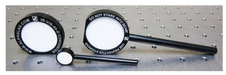
he IR-VIS series from ALPHALAS are unique infrared-to-visible converters suitable for CW and pulsed IR laser sources as well as IR laser diodes. They are ideally suited for tasks like detecting invisible IR radiation, identifying mode structure, etc. Therefore, the visualizers are indispensable tools for every laboratory using Nd:YAG or other IR lasers.
