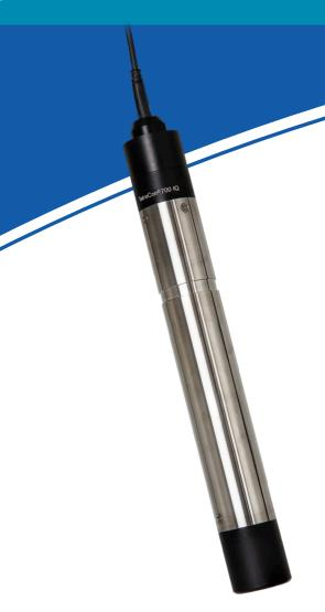
**The TetraCon® submersible conductivity probe** is a rugged electrode-style conductivity probe for the IQ SensorNet process monitoring system. The TetraCon provides continuous and reagentless monitoring of conductivity, salinity, or total dissolved solids (TDS) using a 4-electrode measuring cell to eliminate polarization effects and reduce measurement error due to fouling.
