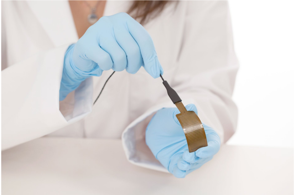
Figure 2.2 Heat flux from the back side to the front side generates a positive voltage output signal. The dot on the foil indicates the front side.
