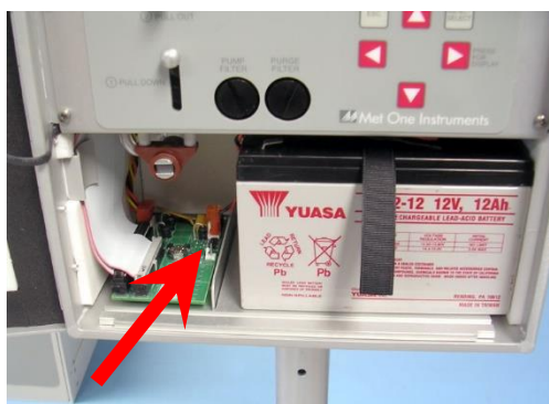
Internal battery and 81220 PCB battery harness connection
