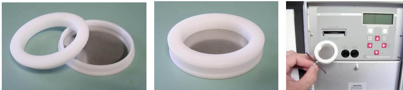
The 47 mm Filter Cassette and Filter Tray
