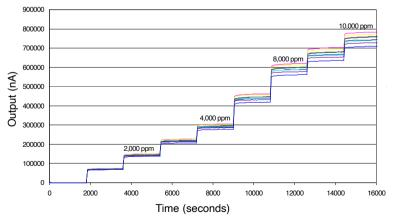
Figure 3 shows the response for a batch of sensors to high concentrations of SO<sub>2</sub> applied as sequential step increases.
