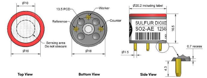
Dimensions are in millimetres (± 0.1 mm).
