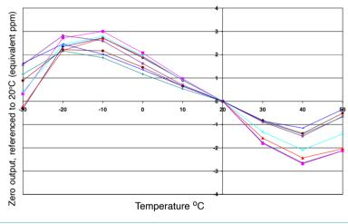
Figure 2 shows the variation in zero output caused by changes in temperature, expressed as ppm gas equivalent, referenced to zero at 20°C. This data is taken from a typical batch of sensors.
