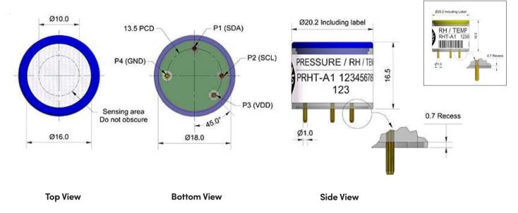
Dimensions are in millimetres (± 0.15 mm).
