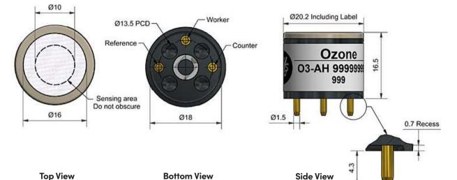
Dimensions are in millimetres (± 0.15 mm).
