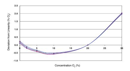
Mass flow oxygen sensors generate a non-linear current with increasing oxygen concentration: current = k \* log (1/(1-C)).
