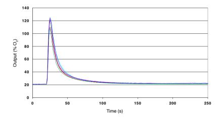
Step changes in pressure can cause a temporary signal transient. Positive pressure gives an output signal increase whilst negative pressure causes the output signal to decrease.
