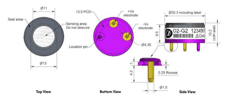
Dimensions are in millimetres (± 0.15 mm).
