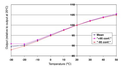
Figure 1 shows the variation of sensor output in clean air due to temperature changes.
