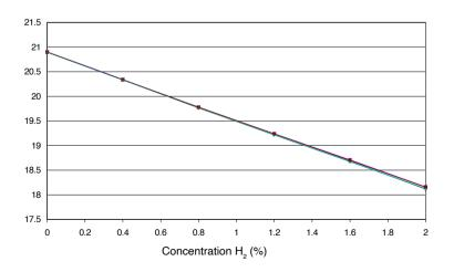
Hydrogen reduces the oxygen sensor output by 6.5%.
