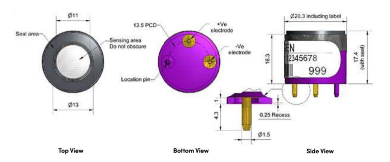
Dimensions are in millimetres (± 0.15 mm).
