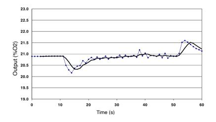
Many gas detectors use either pumps or hand aspirators to sample gases remotely. Pressure transients, caused by pumping, can set gas detectors into alarm.
