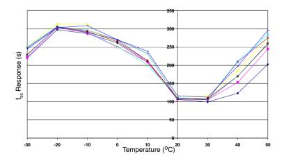
The response time depends on both gas properties and sensor electrochemistry.
