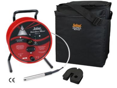
If there is only water in the well and no product, there will only be intermittent (water) signals. The presence or absence of dense (sinking) non-aqueous layers (DNAPL) is determined by continuing to lower the probe to the bottom of the well.
