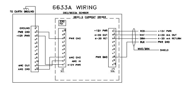
Figure 3.6 – 6633A Wiring
