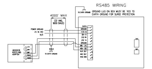
Figure 3.4 – RS485 Wiring
