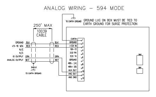
Figure 3.2 – Analog Wiring (594 Mode)
